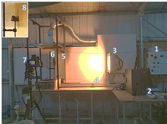
**Fig. 1** Configuration of VHFlux apparatus. (1) Switchboard, (2) PC control system, (3) radiative panel, (4) linear stage, (5) shutter, (6) rotisserie to hold Banksia cones, (7) thermal imaging camera for observation purposes, and (8) stage to hold Hakea cones
