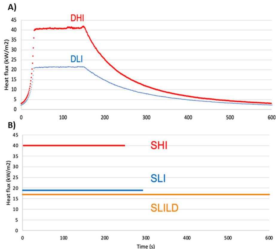
**Fig. 2** Fire intensity treatments. The x-axis displays the time in seconds and the y-axis displays the radiative heat flux in kilowatts per square meter. **A** Dynamic heat treatments, displaying changes in heat flux over time. These include dynamic high intensity (DHI) and dynamic low intensity (DLI). **B** Static heat treatments, displaying a constant heat over time. These include static high intensity (SHI), static low intensity (SLI), and static low intensity long duration (SLILD)
