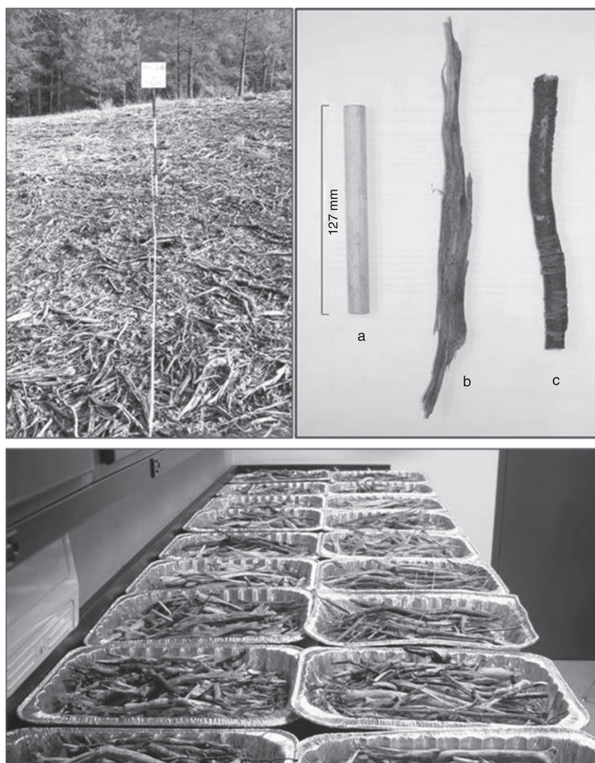
Fig. 1. Photographs of: the masticated fuelbed at the Mad River fuelbreak, Six Rivers National Forest, California (upper left); examples of a dowel ( a ), fractured ( b ) and intact ( c ) particle (upper right); and the constructed experimental fuelbeds used to quantify moisture dynamics in masticated fuelbeds (bottom).
