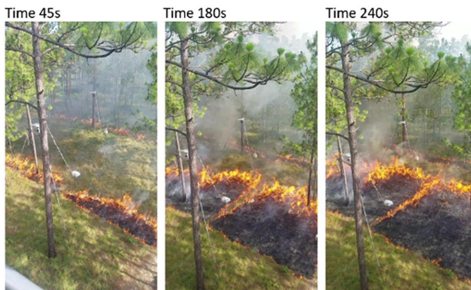
Fig. 3. A simplified ignition pattern of 2 head fires illustrates WFE influences on fire spread over the course of 4 minutes. First, the upwind ignition line entrains ambient flows, stalling the forward spread of the downwind line (seen by the much greater spread distance of the upwind fire in the foreground compared with the downwind fire in the background). Further, a fine-scale discontinuity of fuels creates a break in the upwind fire that develops into a seam between two flanking fires. As the upwind fire line continues to spread as a head fire with the ambient wind, the entrainment patterns of the flanking fires draw them together, spreading perpendicular to the direction of ambient flow (photos by J. O'Brien).
