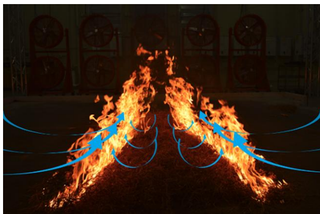
Fig. 4. Illustration of WFE-induced draw between two flanking fire lines (these lines are parallel to each other and the line of sight through the middle of the image, even though the parallax makes them appear as though they converge). When two fires are within the L_E of each other, the competition between WFE from the two fires in the space between them limits the strength of entrainment into either fire from the interior space. The entrainment from the exterior spaces (left and right of the fire lines, respectively) can become stronger than the entrainment to either fire line from the interior space (photos by J. O'Brien).
