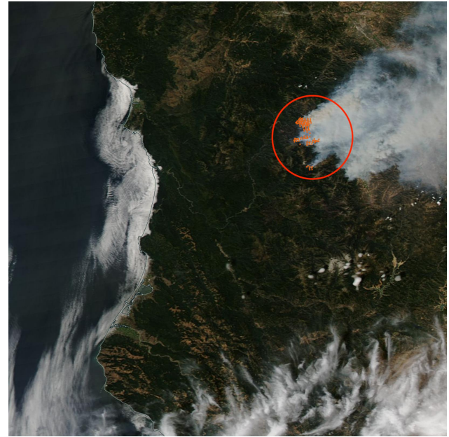
Fig. 6. Visual satellite image of the Happy Camp fire on 29 August 2014, from NASA WorldView. Orange circles represent MODIS thermal anomalies, showing the location of the fire (the area of interest is denoted by a larger red circle). This is an example of a clear day with no satellite remote sensing issues in the FEI.
